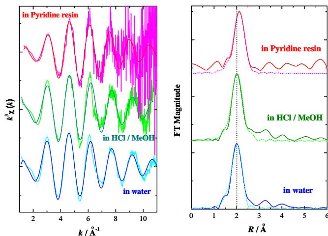
Fig. 1 Nd-L<sub>III</sub> EXAFS and corresponding Fourier transforms for solution samples and resin sample.
